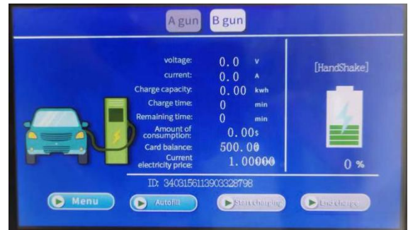
4. Automatic pre-charge check
